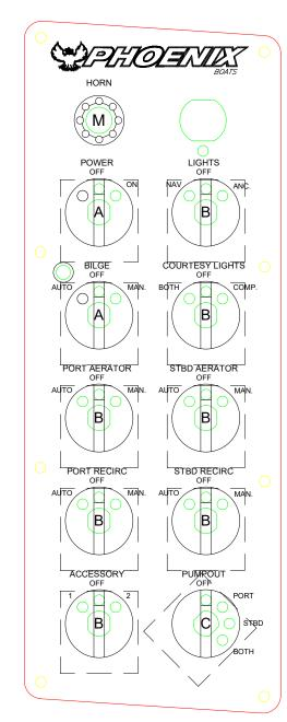
A - ON/OFF SWITCH B - ON/OFF/ON SWITCH C - OFF/1/2/BOTH SWITCH
