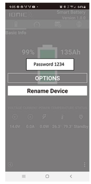
When you get your batteries, Install the app on your phone called Ionic Blue, when you first open the app if it ask do you want to allow location or gps say YES, separate the batteries one at a time, open the app, click the link to connect to that battery, at the bottom of the screen, click the 3 dots, enter password 1234
